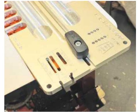
▲ Indexing shoes and slots along with etched lettering make it easy to set positions
